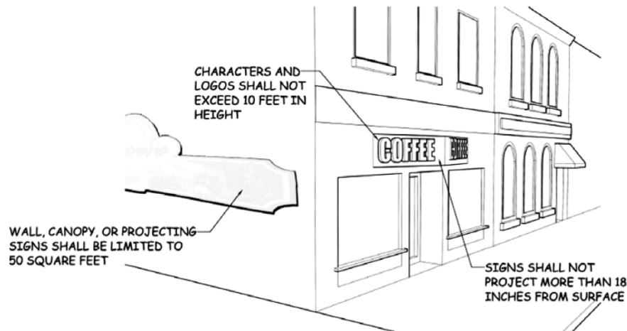
Figure 5.9-2: Example of wall and canopy signs.
